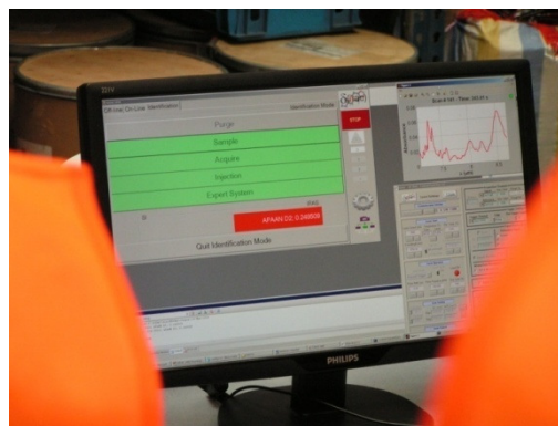
Fig. 6: DIRAC demonstration. Left: liquid traces of precursor in ethanol, collected on a swab, are loaded into the thermal desorber. Right: the system correctly identifies the target.
